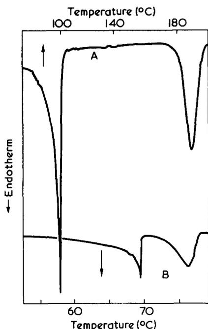
*Figure 1* Thermograms of ionic complexes of poly(ethylene oxide). A, Sodium iodide/PEO 600 000 (crystallized from solution); B, ammonium thiocyanate/PEO 6000 (crystallized at 51°C)
